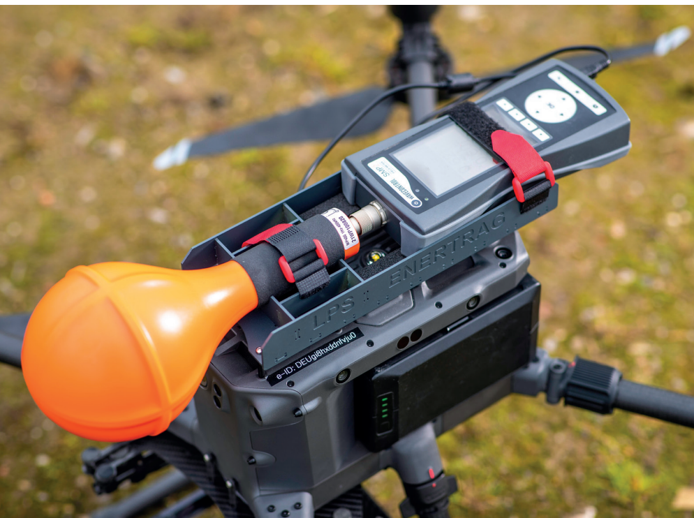
Close-up of a drone for rotor blade inspection and lightning protection measurement. In focus: the field strength meter for testing lightning protection
